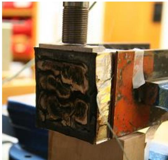
Loading of specimen with visible smouldering (right)
