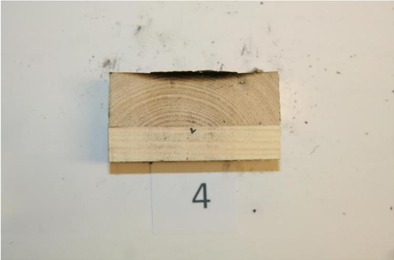
Test specimen no.4 after failure. Bond line failure
