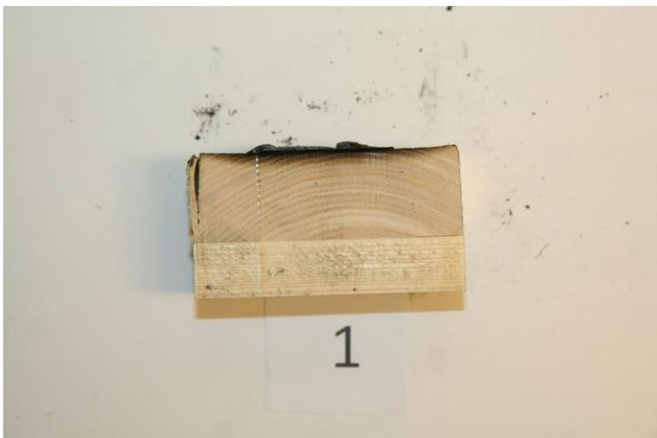
Test specimen no.1 after failure. Partial char and bond line failure.
