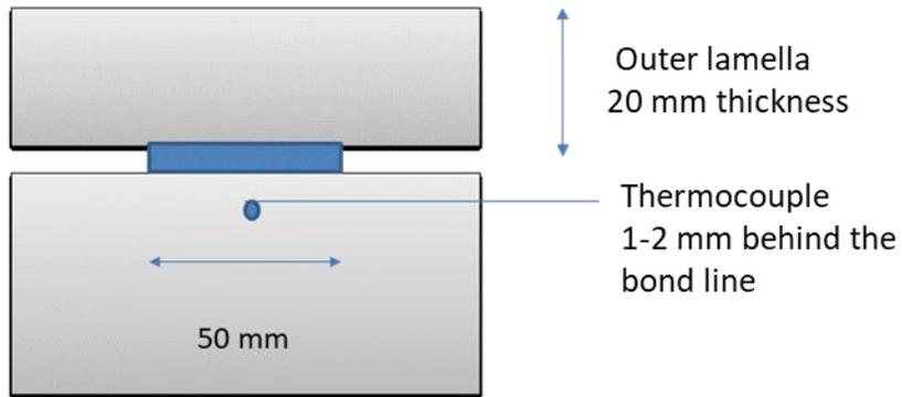
Figure 2. Small scale CLT specimen for fire testing without gypsum board protection
