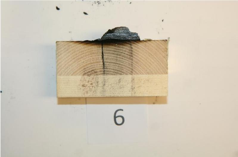
Test specimen no.6 after failure. Char failure.
