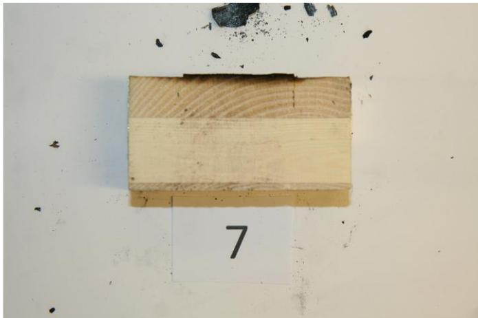
Test specimen no.7 after failure. Bond line failure.
