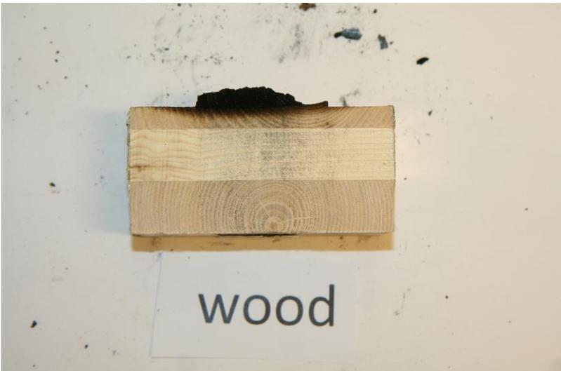
Test specimen without glue line after failure. Char failure.
