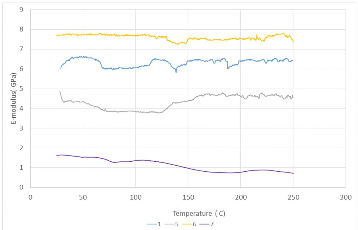
Figure 7 Modulus of elasticity in temperature scan measured by DMA.
