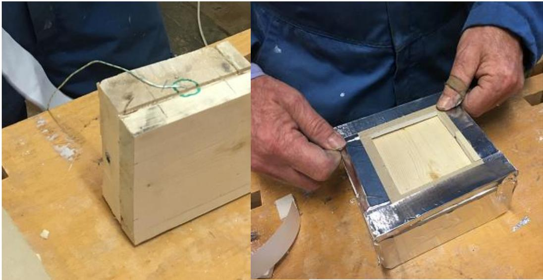
Figure 3. Left – Insertion of thermocouples to the bond line; Right – Application of gypsum plasterboards to the sides of timber specimen.
