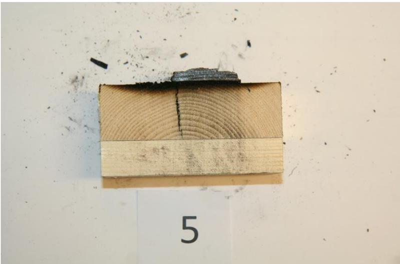
Test specimen no.5 after failure. Char failure.
