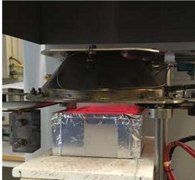
Figure 4. Fire testing with cone heater.
