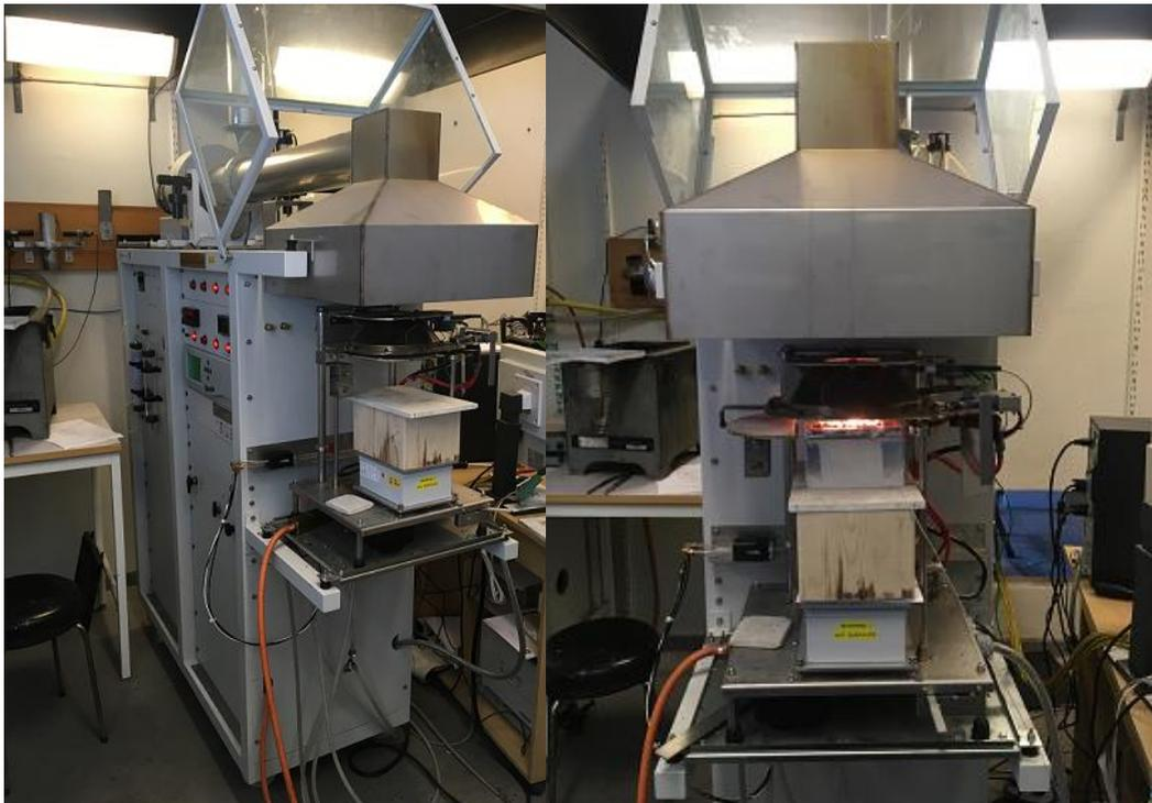
Figure 1. Cone calorimeter (left)
