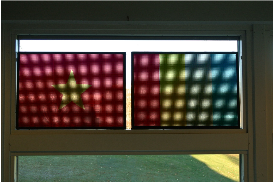
Figure 18: Examples of colored semi-transparent CIGS PV modules developed by Solibro Research [18]. The PV modules are seen from the inside to out.
