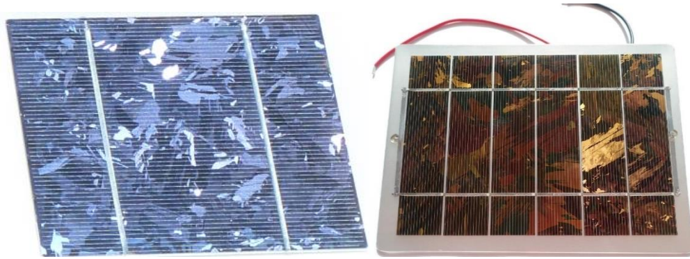
Figure 8: Left: multicrystalline Si solar cell in its original colour; right: multicrystalline Si solar cell with modified thickness of AR COATING (on top of semiconducting material) from Solar Capture Technologies ( www.solarcapturetechnologies.com ).
