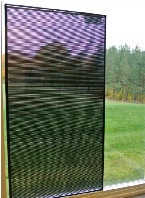
Figure 13: CIGS solar cell with removed semiconductor material using dry sand-blasting achieving 40% transparency - this is not yet a certified product (Source: Neretnieks, P. Utveckling av semitransparenta solpaneler. in Solforum. 2017. Västerås, Sweden.)
