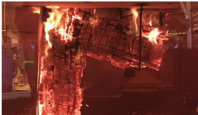
Figure 11: Connection 2 fire test 6 minutes after failure
