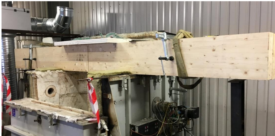
Figure D3. Preparation for the fire test of the moment connection.
