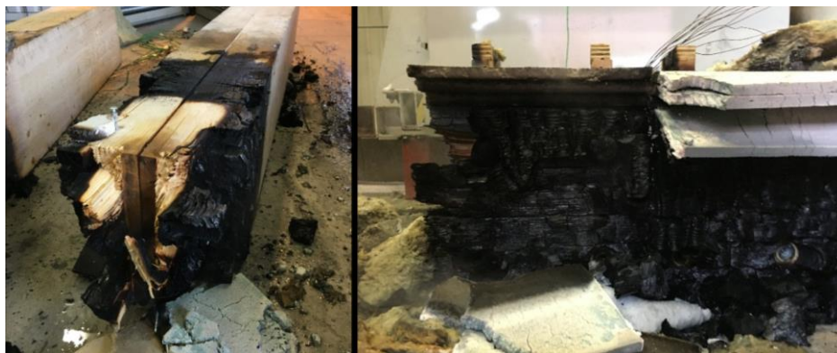
Figure 16: Specimen after the fire test – failure mode: bending failure at the minimum cross-section
