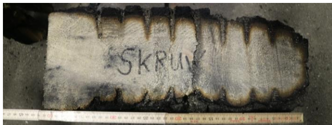
Figure 7: Photo of cross-section of beam with charred screw holes.
