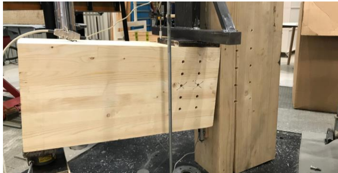
Figure 10: Connection 1 after room temperature test
