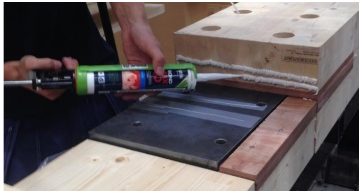
Figure 15: Two strips of fire sealant at the gap.
