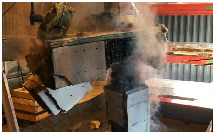
Figure 13: Specimen after the fire test (end support failed)
