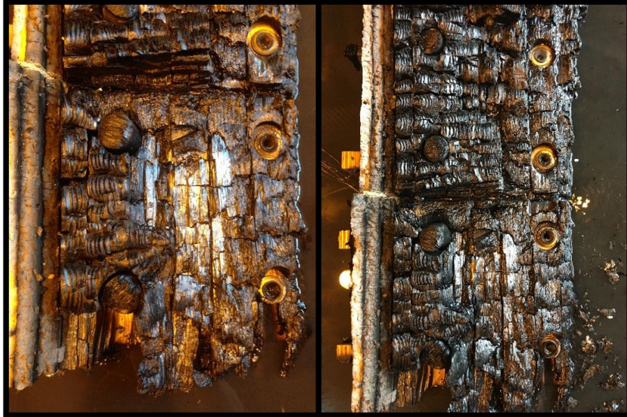
Figure D7. Tubes after the test without a sign of damage
