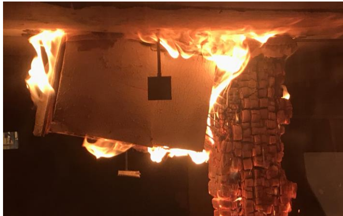
Figure 6: Connection 1 fire test 10 minutes after failure
