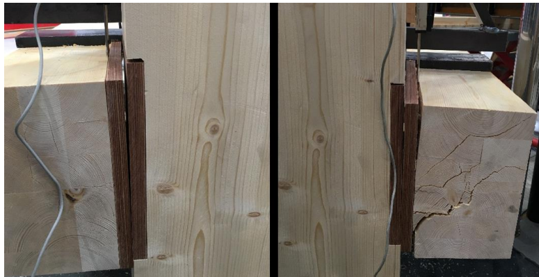
Figure C3: the failure mode for high shear forced.
